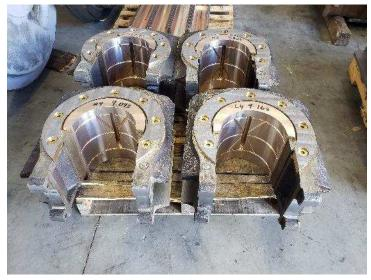
The photo on the left are parts of the shoes and wedges that the drive boxes ride in. On the right are the crown brasses set in the drive boxes. There are eight total crown brasses and drive boxes. The drive boxes are original to the locomotive. The crown brasses are designed to be replaced as they wear out. The eight crown brasses are all new and the all eight drive boxes have been refurbished.
