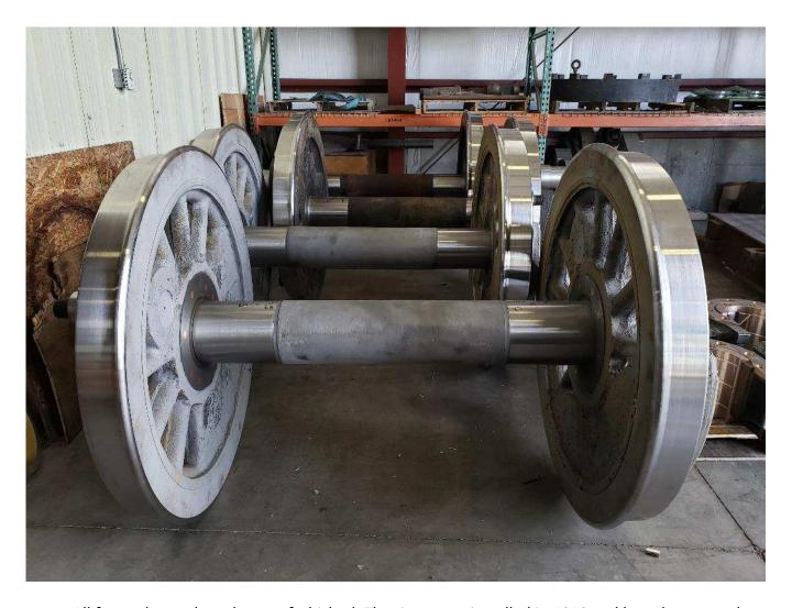
All four axle sets have been refurbished. The tires were installed in 1949 and have been trued up. The shiny areas on the axles are where the crown brasses will ride.
