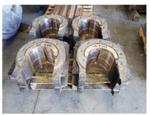
The photo on the left are parts of the shoes and wedges that the drive boxes ride in. On the right are the crown brasses set in the drive boxes. There are eight total crown brasses and drive boxes. The drive boxes are original to the locomotive. The crown brasses are designed to be replaced as they wear out. The eight crown brasses are all new and the all eight drive boxes have been refurbished.
