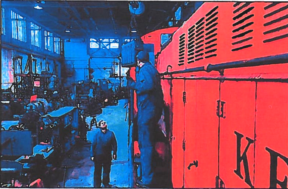
The first of sixteen batteries is being installed into Locomotive 81. There will be eight batteries per side. Each battery weighs 300 pounds.
