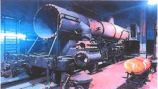
The locomotive is essentially stripped down to almost nothing. Our plan is to remove the pilot truck in the coming month.
