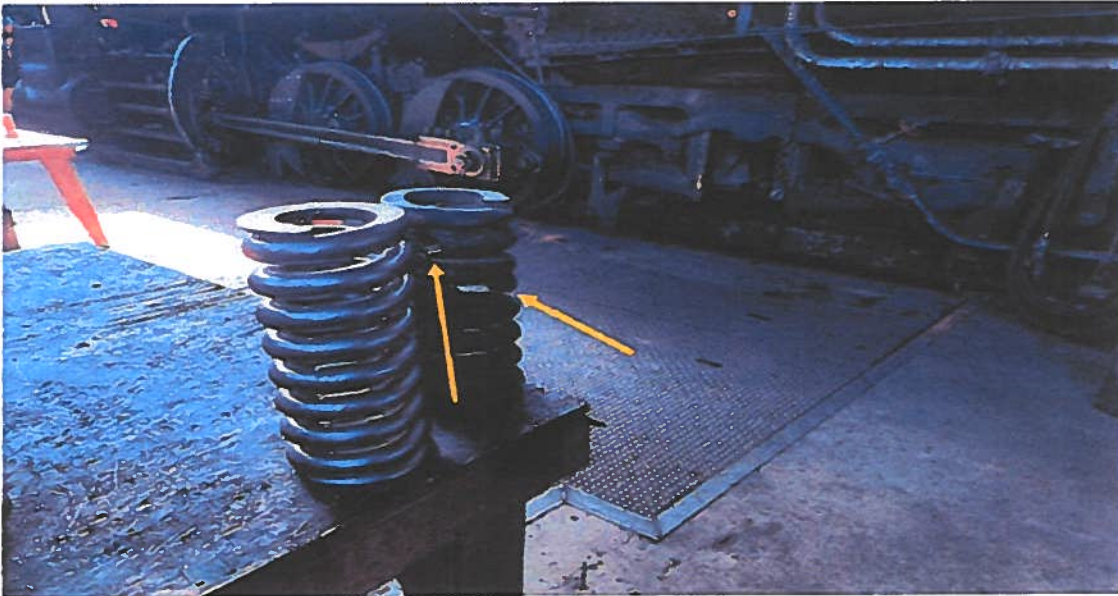
The yellow arrows point to the breaks in the spring. We were able to custom springs created to replace the broken ones and to have a few spares too.
