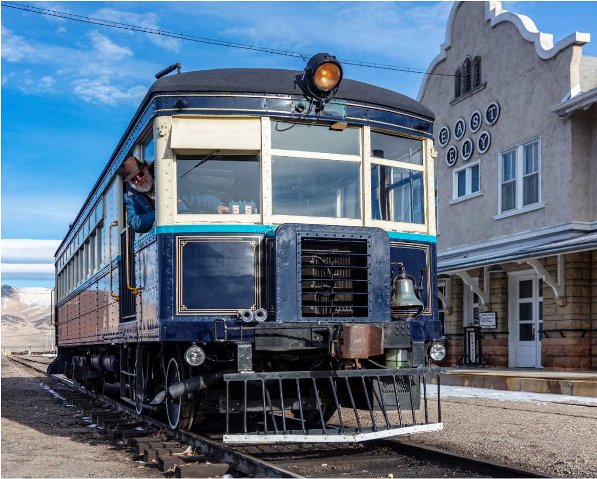
The car is powered by a Chevy 396 CI V-8 and can carry 40 passengers.
