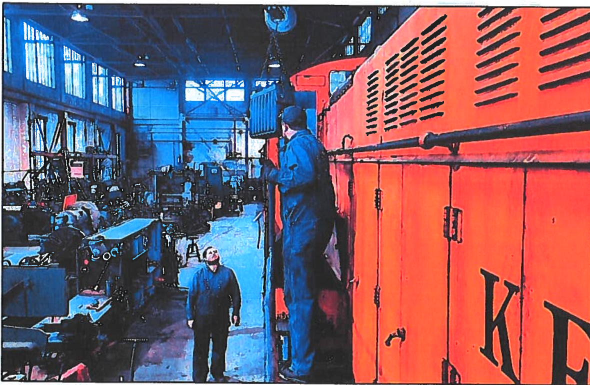
The first of sixteen batteries is being installed into Locomotive 81. There will be eight batteries per side. Each battery weighs 300 pounds.
